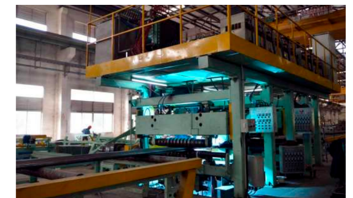
Membrane wall welding production line
