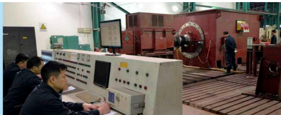
Type test of end cap bearing motor in the workshop
